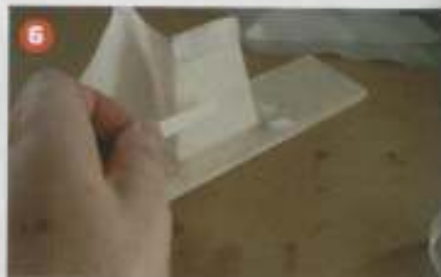
PHOTO 6: The glass-cloth is applied using small plastic strips.
